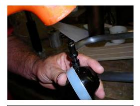
Step 5: Place ferrule end of new pin in caster hole and tap pin into place with rubber of plastic mallet.
