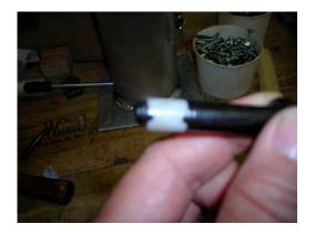
Step 4: Place a new white plastic ferrule on a new caster pin.
