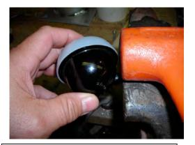
Step 2: Using a rubber or plastic mallet, gently strike caster to remove it from the existing pin.
